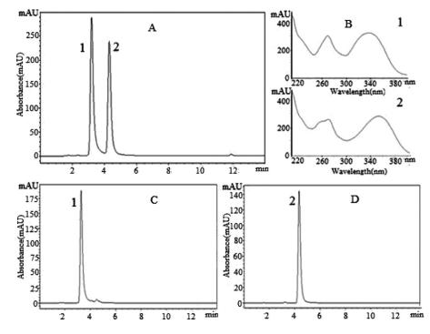
**FIGURE 3** HPLC chromatogram of crude sample (A), lutonarin (C), and saponarin (D) and UV spectrum of lutonarin and saponarin (B); lutonarin (1) and saponarin (2); Column: Eclipse XDB  $C_{18}$  column (250 mm × 4.6 mm I.D., 5 µm); mobile phase: methanol and water in gradient mode (methanol: water (v/v) from 38: 62 to 62: 38, in 13 min); flow rate: 1.0 mL min<sup>-1</sup>; detection wavelength: 270 nm; column temperature: 30°C.
