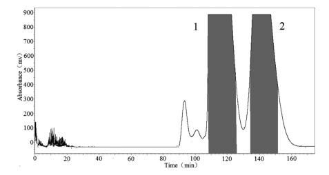
**FIGURE 2** HSCCC chromatogram of crude extract from Barley seedlings. Two phase solvent system: ethyl acetate/*n*-butanol/water 3:2:5, v/v/v; mobile phase, the lower phase; flow rate 1.6 mL min<sup>-1</sup>; revolution speed, 900 rpm; detection wavelength, 280 nm; separation temperature, 25°C; sample size, 100 mg sample dissolved in 20 mL of the lower phase. Retention of the stationary phase: 42%.
